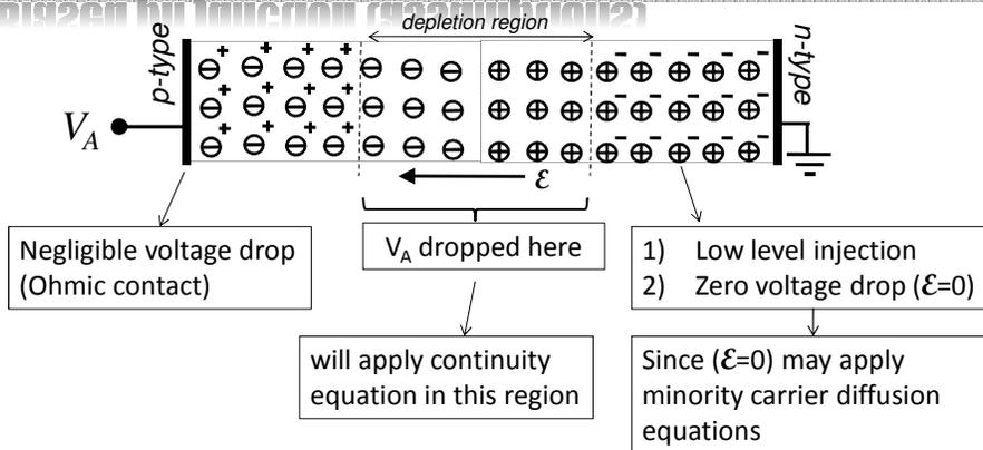
Note:  $V_A$  should be significantly smaller than  $V_{bi}$  (Otherwise, we cannot assume low-level injection)
