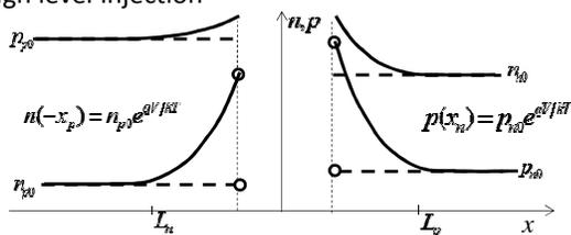
In High level injection condition we should add recombination current to the continuity equations from the minority carriers, result will be as:
