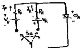
$$@t = 0^- (V_F \gg V_A) \rightarrow I_F = \frac{V_F}{R_F} \quad (\text{as } V_A < .7v)$$
