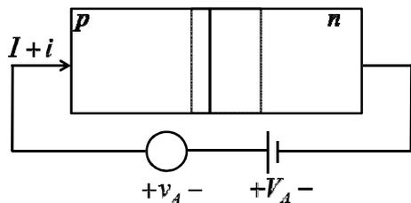
A small ac signal ( $v_a$ ) is superimposed on the DC bias. This results in ac current ( $i$ ). Then, admittance  $Y$  is given by
