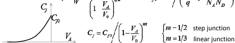
$$C_j = C_{j0} / \left(1 - \frac{V_A}{V_0}\right)^m \quad \begin{cases} m = 1/2 & \text{step junction} \\ m = 1/3 & \text{linear junction} \end{cases}$$
