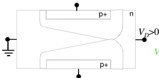
$$V_{Dsat} = V_G - V_P = V_G - \phi_0 + \frac{qN_D a^2}{2\epsilon}$$
