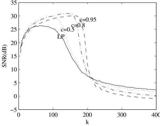
Fig. 6. Averaged SNR's (over 100 runs of the algorithm) versus  $k$ , the average number of active sources, for SL0 algorithm with several values of  $c$ , and for LP. The parameters are  $m = 1000$ ,  $n = 400$ ,  $\sigma_1 = 1$ ,  $\sigma_J = 0.01$ ,  $\sigma_n = 0.01$ .
