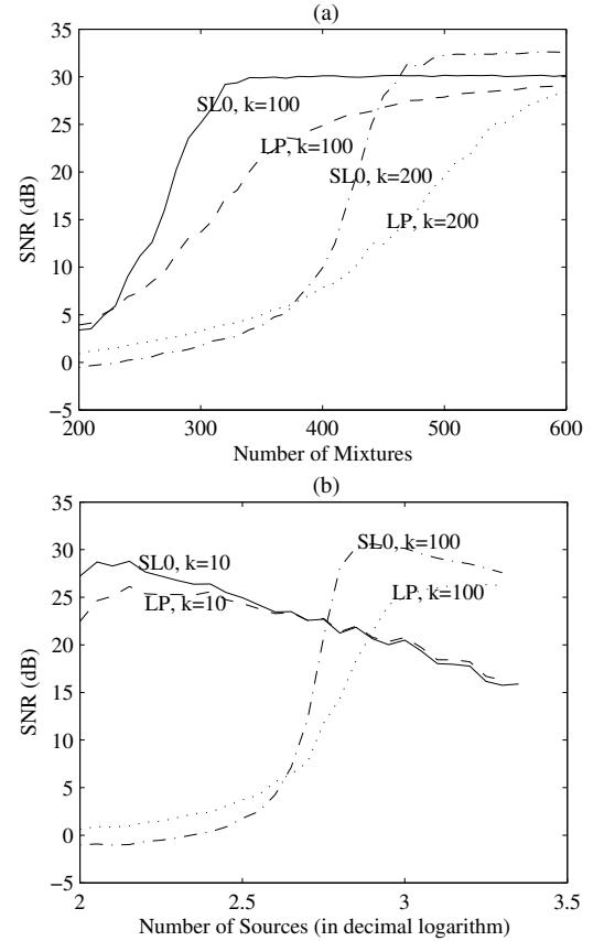
Fig. 8. Effect of scale on performance (SNR's are averaged over 100 runs of the algorithm).  $\sigma_n = 0.01$ ,  $c = 0.8$ ,  $\sigma_1 = 1$ ,  $\sigma_J = 0.01$ , and SL0 is compared with LP. In (a)  $m$  is fixed to 1000 and SNR is plotted versus  $n$  for different values of  $k$ . In (b) SNR is plotted versus  $\log(m)$  for different values of  $k$ , while  $n$  is fixed to  $[0.4m]$ .
