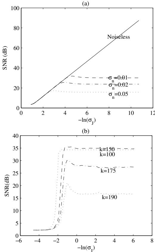
Fig. 4. Performance of SL0 versus  $\sigma_J$  for  $m = 1000$  and  $n = 400$  (SNR's are averaged over 100 runs of the algorithm).  $\sigma_1$  is fixed to 1 (large enough) and  $c$  is fixed to 0.8 (near enough to one). In (a)  $k$  is fixed to 100 and effect of noise is investigated. In (b)  $\sigma_n$  is fixed to 0.01 and effect of sparsity factor is analyzed.
