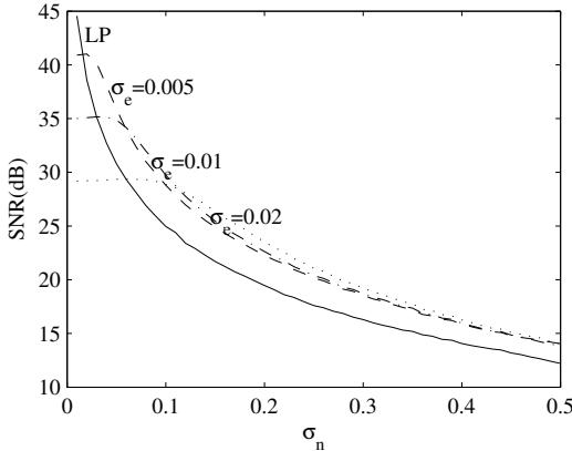
Fig. 7. Averaged SNR's (over 100 runs of the algorithm) versus the noise power  $\sigma_n$  for different values of  $\sigma_J$ , and for LP. The parameters are  $m = 100$ ,  $n = 400$ ,  $k = 100$ ,  $\sigma_1 = 1$ , and  $c = 0.8$ .
