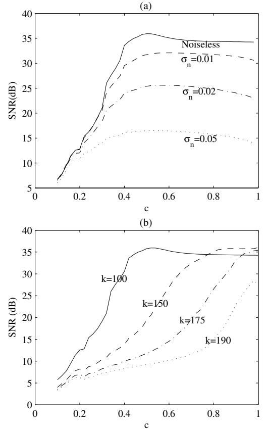
Fig. 3. Performance of SL0 as function of  $c$  for the case  $m = 1000$  and  $n = 400$  (SNR's are averaged over 100 runs of the algorithm).  $\sigma_1$  is fixed to 1 (large enough) and  $\sigma_J$  is fixed to 0.01 (small enough). In (a)  $k$  is fixed to 100 and effect of noise is investigated. In (b)  $\sigma_n$  is fixed to 0.01 and effect of sparsity factor is analyzed.
