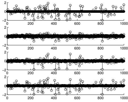
Fig. 2. Evolution of SL0 toward the solution:  $m = 1000$ ,  $n = 400$  and  $k = 100$  ( $p = 0.1$ ). From top to bottom, first plot corresponds to the actual source, second plot is its estimation at the first level ( $\sigma = 1$ ), third plot is its estimation at the second level ( $\sigma = 0.5$ ), while the last plot is its estimation at third level ( $\sigma = 0.2$ ).
