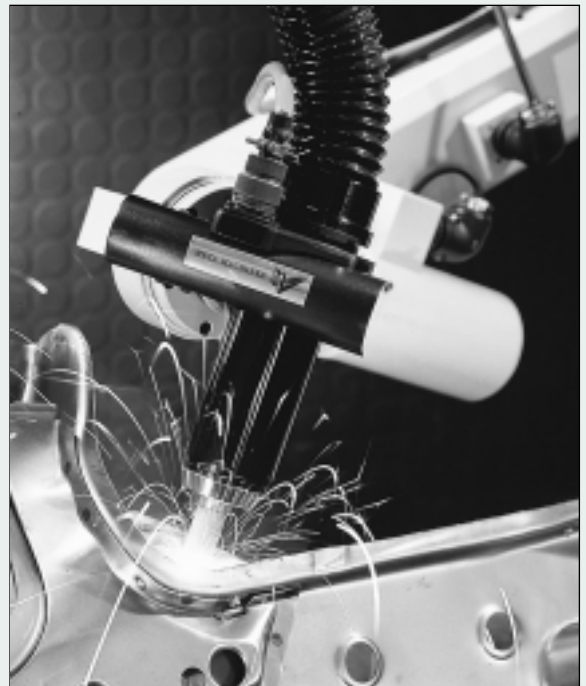
A welding robot. (Courtesy of Shela Terry/Science Photo Library.)
