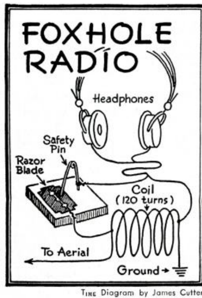
Figure 1: Foxhole radio as published in Time magazine.
