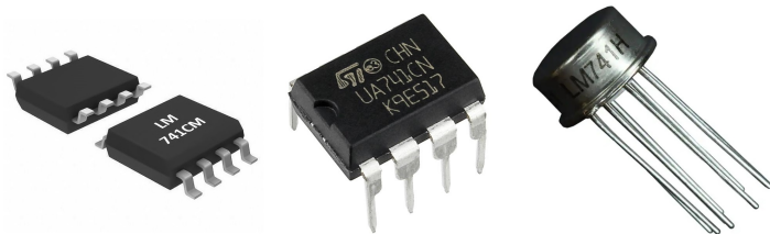
Figure: Single op-amp LM741 IC in SMD and through-hole packages.
