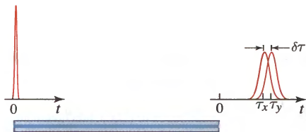
Figure: Differential group delay associated with polarization mode dispersion (PMD). PMD appears since the fiber is not perfectly circular and isotropic.
