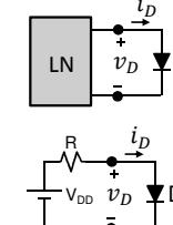
$$V_{DD} = 5V, R = 1k\Omega, I_s = 5 \times 10^{-14}A, V_T = 26mV$$
