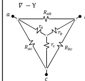
$$\begin{aligned} r_a &= \frac{R_{ac} R_{ab}}{R_{ac} + R_{ab} + R_{bc}} \\ r_b &= \frac{R_{bc} R_{ab}}{R_{ac} + R_{ab} + R_{bc}} \\ r_a &= \frac{R_{ac} R_{bc}}{R_{ac} + R_{ab} + R_{bc}} \end{aligned}$$
