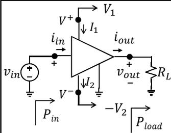
$$\left\{ \begin{array}{l} V_{1,2} = \pm 10V \\ I_1 = 9.5mA \\ v_{in} = 1^V \sin \omega t \\ i_{in} = 0.1mA \sin \omega t \end{array} \right. \quad \left\{ \begin{array}{l} I_2 = 9.5mA \\ v_{out} = 9^V \sin \omega t \\ R_L = 1^k\Omega \end{array} \right.$$
