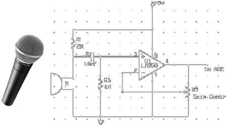
Output voltage of a sensor → Amplifier → Process
