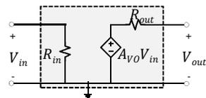
$$A_{vo} = \frac{V_{out}}{V_{in}} \Big|_{i_{out}=0}$$
