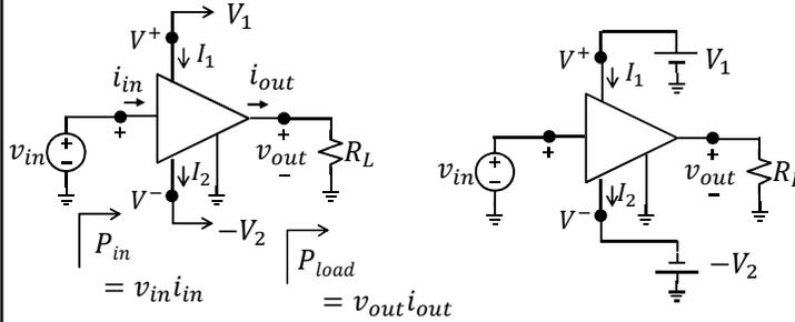
$$P_{dc} = P_{supply} = V^+ I_1 - V^- I_2 = V_1 I_1 + V_2 I_2$$
