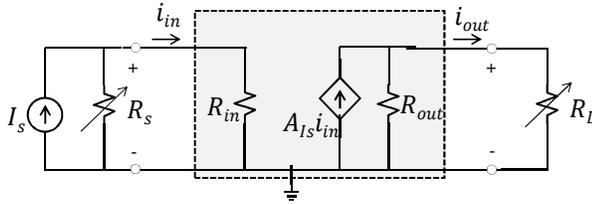
Short circuit:  $R_L = 0 \rightarrow \frac{i_{out}}{i_{in}} = A_{I_s} \left[ \frac{A}{A} \right]$  short circuit current gain
