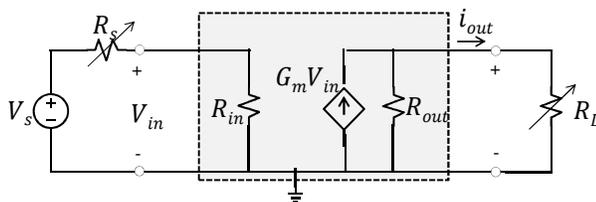
Short circuit:  $R_L = 0 \rightarrow \frac{i_{out}}{V_{in}} = G_m \left[ \frac{A}{V} = \Omega^{-1} \right]$  short circuit Trance-conductance
