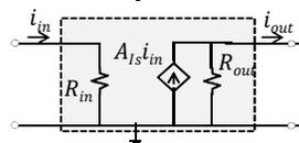
$$A_{is} = \frac{i_{out}}{i_{in}} \Big|_{v_{out}=0}$$
