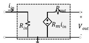
$$R_m = \frac{V_{out}}{i_{in}} \Big|_{i_{out}=0}$$
