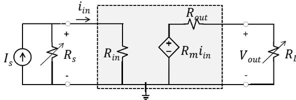
Short circuit:  $R_L = \infty \rightarrow \frac{V_{out}}{i_{in}} = R_m \left[ \frac{V}{A} = \Omega \right]$  open circuit Trans-resistance
