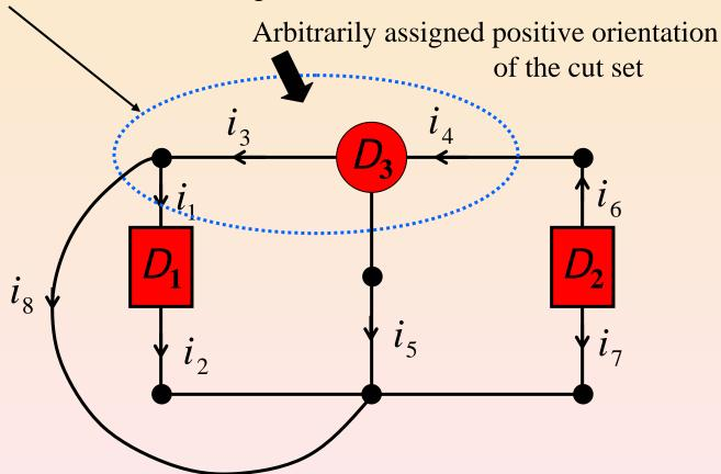
Applying KCL to a Gaussian surface associated with a cut set
