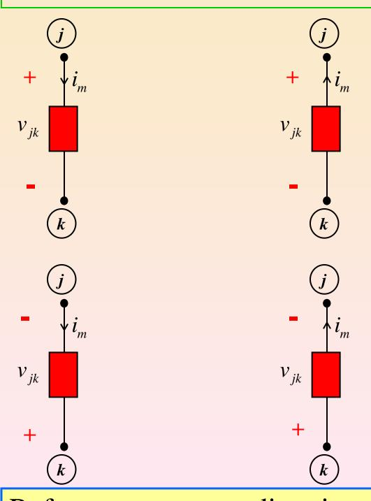
Reference current direction and reference voltage polarity can be arbitrarily assigned.
