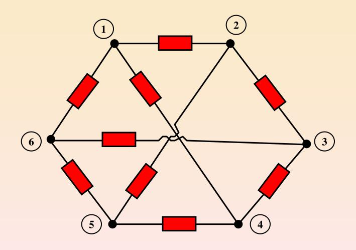
It is impossible to redraw this circuit without intersecting wires.
