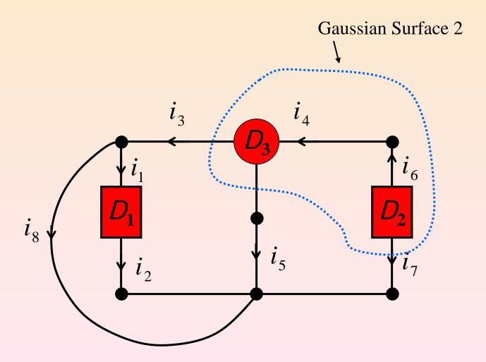
Gaussian Surface 2:  $i_3 + i_5 + i_7 = 0$
