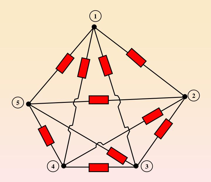
It is impossible to redraw this circuit without intersecting wires.
