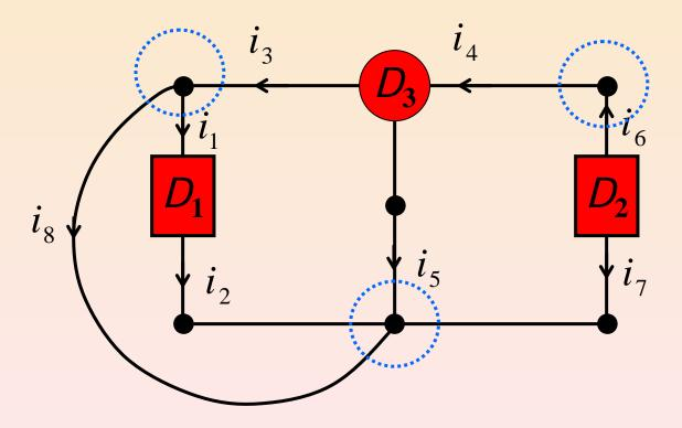
Applying KCL to a small Gaussian surface enclosing each node
