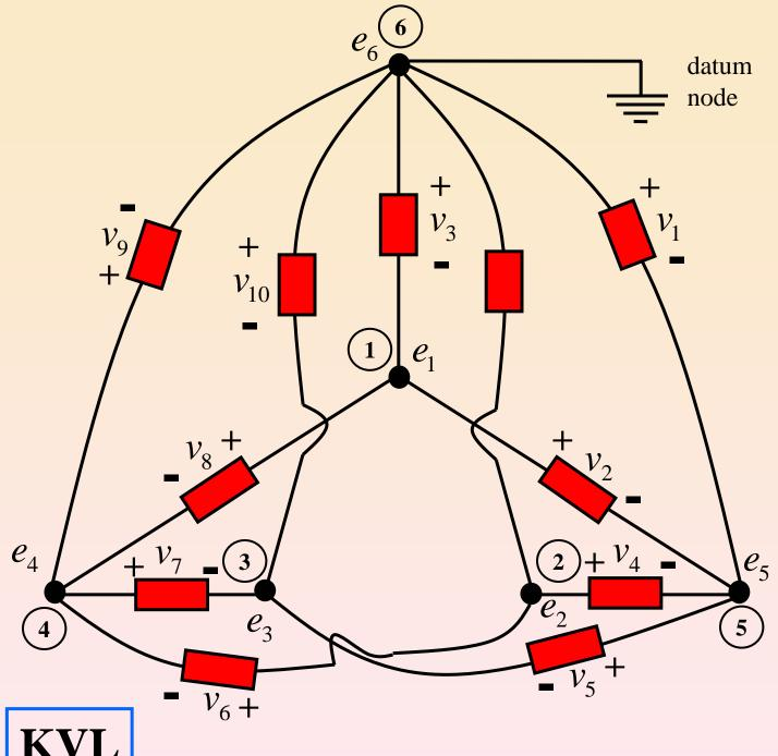
$$v_1 = e_6 - e_5 = -e_5, \ v_4 = e_2 - e_5$$
