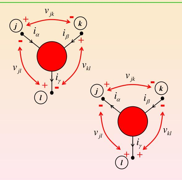
Note: When two terminals whose voltage polarity is being assigned are far apart, we often draw a double-headed arrow to identify the associated pair of terminals.
