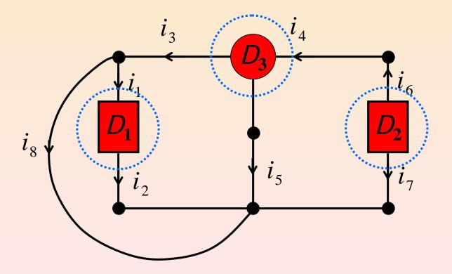
Applying KCL to a Gaussian surface enclosing each device ⇒
