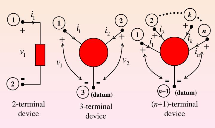
Current is assigned entering the positively referenced non-datum terminal.
