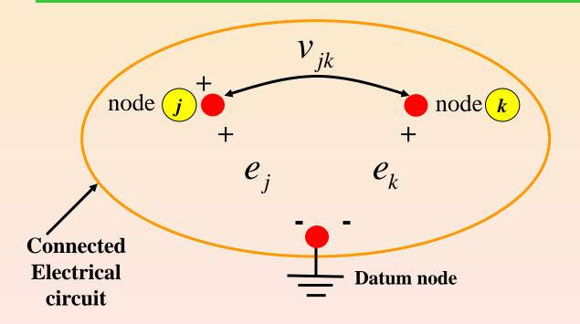
The **voltage**  $v_{jk}(t)$  between *any* 2 **nodes** j
